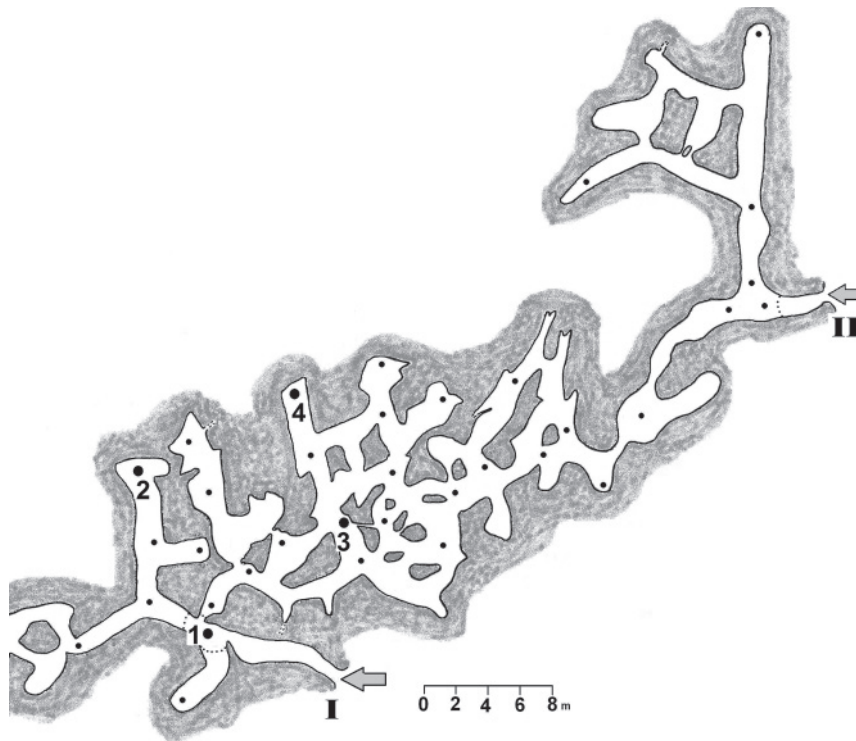
Appendix. Fig. 1. Map of Lipty 1 mine. Large numbered dots — main temperature measurement points (see fig. 1), small dots — additional temperature measurement points. Entrances (numbered I and II) are shown by arrows. The dashed line is the border of the freezing zone.
